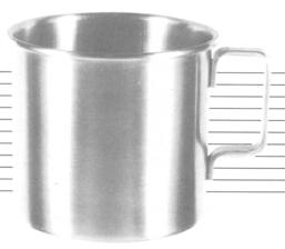
Used in conjunction with AOCS Official Method Ca9a-52 to determine the refining loss of free fatty acids, oil and impurities when the sample is treated with alkali solutions under test conditions. The method applies to crude peanut oil, crude coconut oil, crude corn oil, crude soybean oil (expeller and hydraulic), and crude cottonseed oil (expeller and hydraulic). Cup dimensions: 4 1/2 inch diameter and 4 1/8 inch depth. Capacity: 960 ml.
